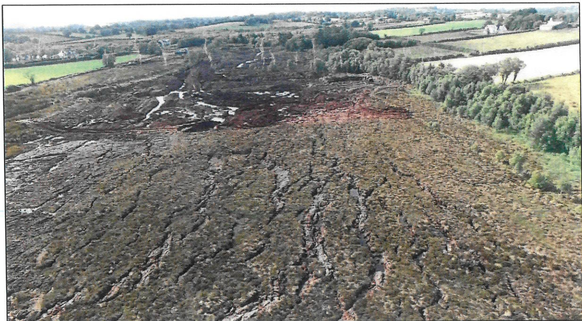
Figure 11: Aerial imagery of proposed unauthorised development. Striations visible in wetland/bog habitat are almost certainly owing to peat shrinkage associated with drainage
